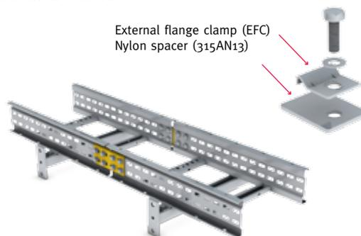
For those installations where it is not practical to fit supports within 600mm on each side of the expansion joint, or for those installations where there is a requirement to provide an expansion coupler capable of accommodating more than 28mm of movement, consideration should be given to the use of the Speedway Full Moment Expansion couplers.
