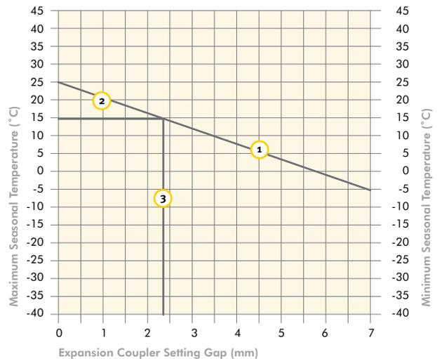
A diagonal line (1) should be constructed between the two vertical axes using the maximum and minimum seasonal temperatures, for example, +25°C & -5°C.
