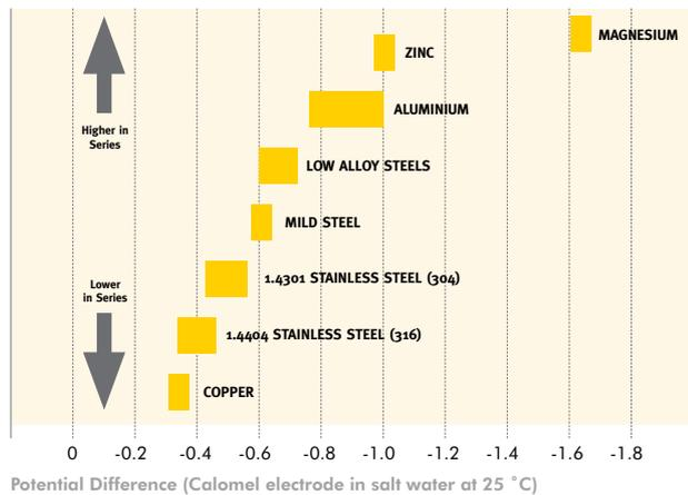
It is common to find dissimilar metals such as stainless steel and mild steel or zinc (as found on a hot dip galvanized item) in contact in a damp atmosphere (i.e. sea water, rain, etc.).
